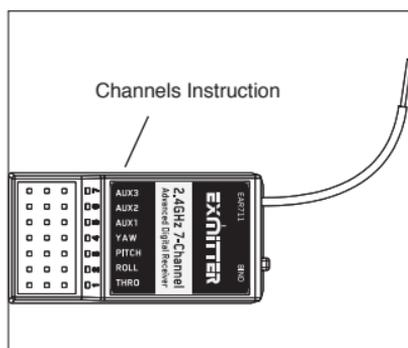
Binding is the process of programming the receiver to recognize the GUID (Globally Unique Identifier) code of a single specific transmitter. When a receiver is bound to a transmitter, the receiver will only respond to that specific transmitter. If you need to rebind for any reason, please follow these steps:
