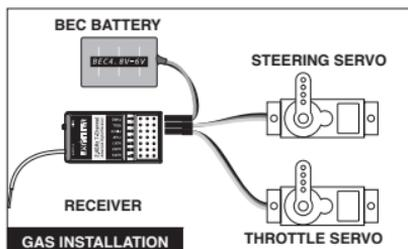
Install the receiver in your vehicle using double-sided Velcro. Velcro will hold the receiver in place and help isolate it from vibrations. Mount the antenna up and away from the vehicle in an antenna tube. The higher up the antenna is, the better signal it will receive.
